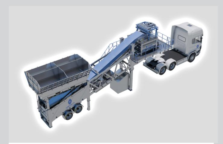
The plant design to produce 3M<sup>3</sup> every 90 sec with a total up to 100M<sup>3</sup> per hour.
